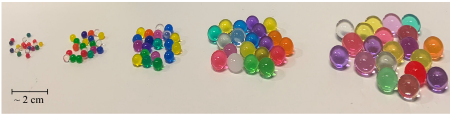
Figure 1. An illustration of different stages of swelling of a super-absorbent gel sold as the children's toy Orbeez™, showing the state in equilibrium with typical indoor conditions on the left and the fully swollen state after immersion in water for some hours on the right.
