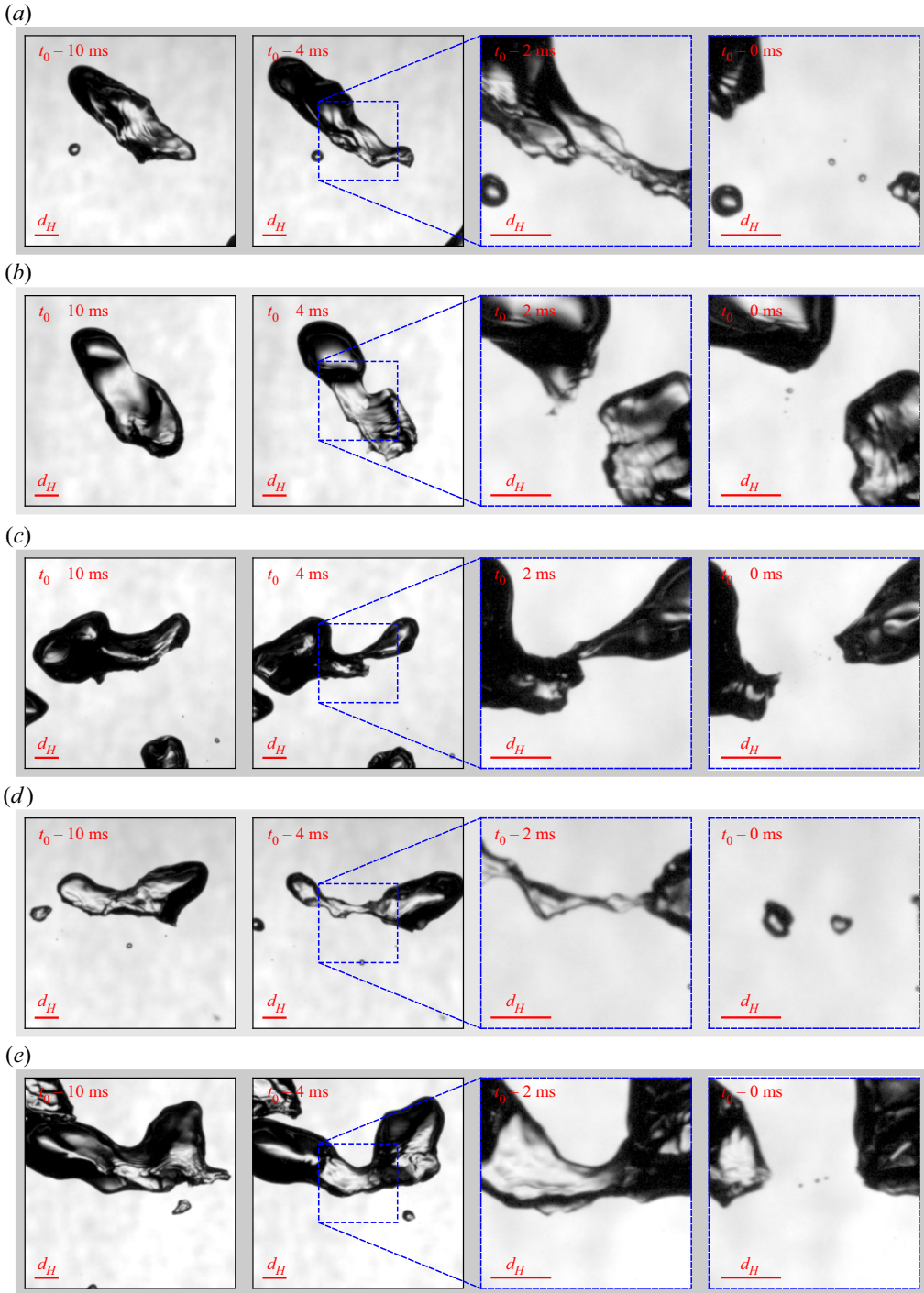
Figure 10. Five cases of sub-Hinze bubble production by the unstable collapse of a deformed ligament. Each row shows four snapshots in time, spaced 10, 4, 2 and 0 ms before the time at which the sub-Hinze bubbles are first visible. The field of view in the final two columns is given by the blue square in the second column. Prior to break-up, the parent bubbles shown are highly deformed, reaching (from the case in the top row to the case in the bottom row) 10.0d_H , 8.7d_H , 8.2d_H , 7.4d_H and 8.0d_H in their longest axis in the images.
