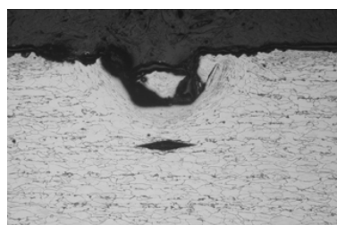
Figures 2 – 4: Cross sections of profiles of threads #3, #8, and #14 (original magnification 100x).
