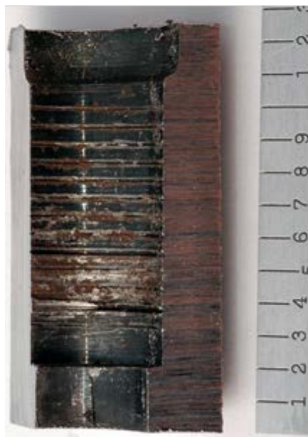
Figure 1: Section of threaded steel region with threads 1-14, top to bottom.
