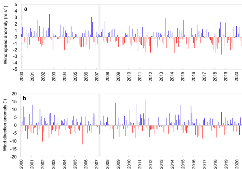
Fig. 10. (a) Mean monthly ERA5-derived wind speed anomalies (deviations from the 2000–2020 monthly mean) extracted over Voyeykov Ice Shelf (red box in Fig. 1). (b) Mean monthly ERA5-derived wind direction anomalies (deviations from the 2000–2020 monthly mean) extracted from the same region. Wind directions vary between 92^\circ (easterly, i.e. blowing from the east) and 122^\circ (south-easterly) over this 20-year period within this region. The period of ice shelf disaggregation is shaded in grey in both plots. Note anomalies calculated over the wider region area (a 26 000 km 2 polygon extending 100 km offshore) were of the same magnitude and variability.
