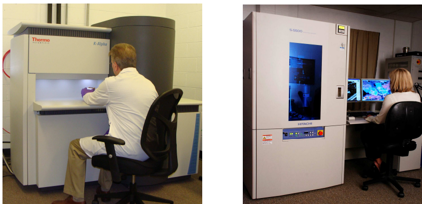
FIG. 3. Thermo Scientific K-Alpha XPS (left) and Hitachi S-5500 30 kV FESEM/STEM (right).
