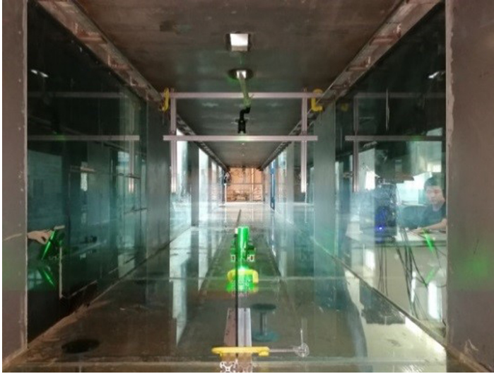
Figure 1. Working section of the wind tunnel taken from the inside.
