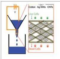
Schematic of the filtration device showing the three components used and the testing technique used for evaluation. NWs is nanowires and CNT is carbon nanotube. Reproduced with permission from *Nano Lett.* **10** (9) (2010) DOI: 10.1021/nl101944e; p. 3628. © 2010 American Chemical Society.
