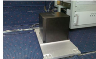
(b) IMU installation
