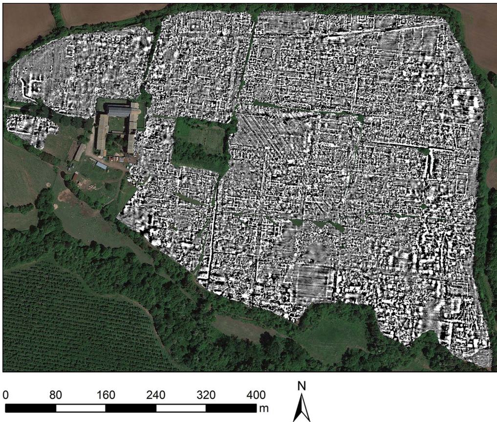
Figure 1. Falerii Novi fluxgate gradiometer survey (Keay et al. 2000); data range -30\text{nT} (white) to +30\text{nT} (black) (aerial photograph: Google Earth; image by L. Verdonck).
