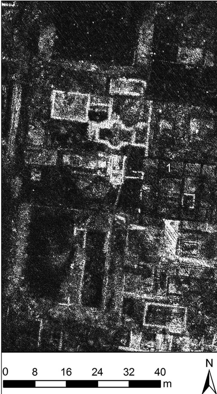
Figure 5. GPR time-slice (case study area), at an estimated depth of 0.75–0.80m (image by L. Verdonck).
