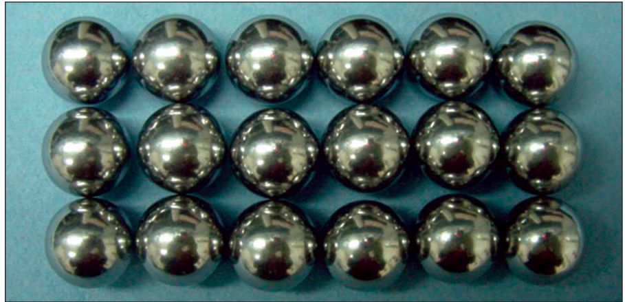
Figure 1. A uniform rhenium coating was applied to 18 graphite balls by placing them into a cylindrical molybdenum wire cage and then rotating the cage in the rhenium vapor above the rhenium melt pool. The diameters of the rhenium-coated balls are ~18 mm.
