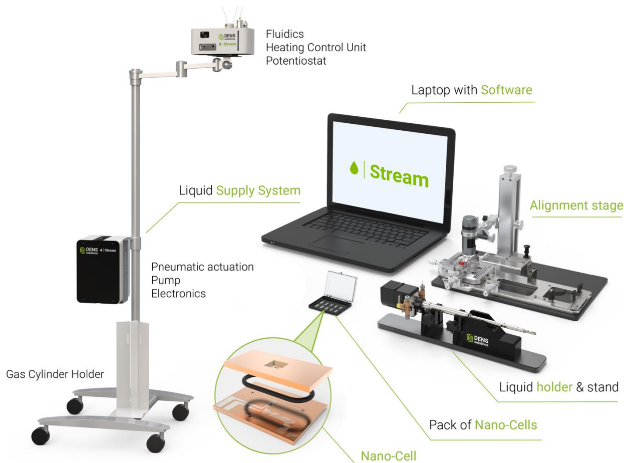
Figure 1. Plug-and-play system for Liquid Phase TEM. In order to enable meaningful experiments, the Nano-Cell (a MEMS-based sample carrier) is inserted into the liquid holder. Once inside the TEM, the user can accurately control pressure, flow rate, liquid thickness using the Liquid Supply System.
