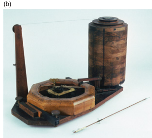
Figure 7.2b Horace Darwin's self-recording auxanometer
