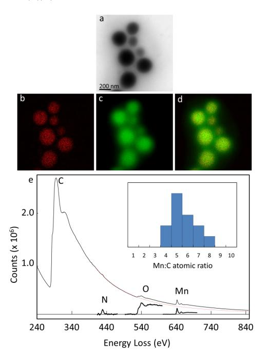
**Figure 1.** EFTEM and EELS analyses of manganese-block copolymer nanocomplexes. (a) TEM image of nanocomplexes, (b) manganese map (red), (c) carbon map (green), (d) overlay of manganese and carbon maps. (e) EELS spectra and background subtracted spectra obtained from the complexes showing the core edge signals of nitrogen (N), oxygen (O) and manganese (Mn). From the spectra the Mn:C atomic ratios were obtained and plotted in the inset histogram.
