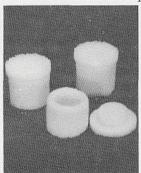
are solvent-resistant (not harmed by alcohol, acetone or chloroform). Capsules can also be used as convenient storage vessels for specimens under desiccation. Outside measures 13mm high by 12mm diameter. Internal storage space is 5mm high by 9mm diameter.
