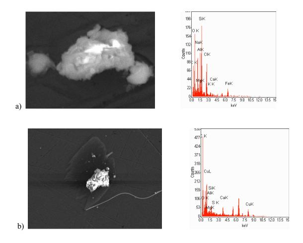
Fig.1.- Image and chemical composition of (a)TSP and (b)PM10 obtained trought SEM
