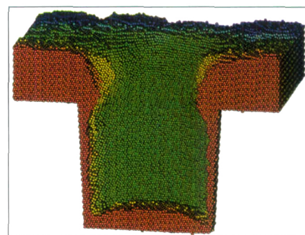
Figure 2. Three-dimensional simulation of copper seed layer step coverage over a sub-micron sized via via ionized physical vapor deposition.
