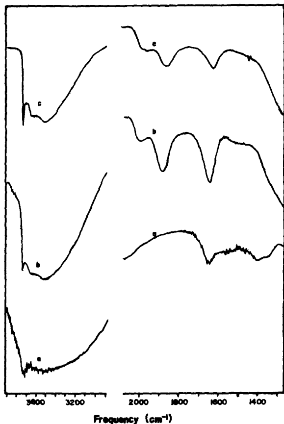
Figure 2. Infrared spectra of adsorbents dried at 120 °C: a) \gamma -alumina; b) silica-gel; and c) Cabosil.
