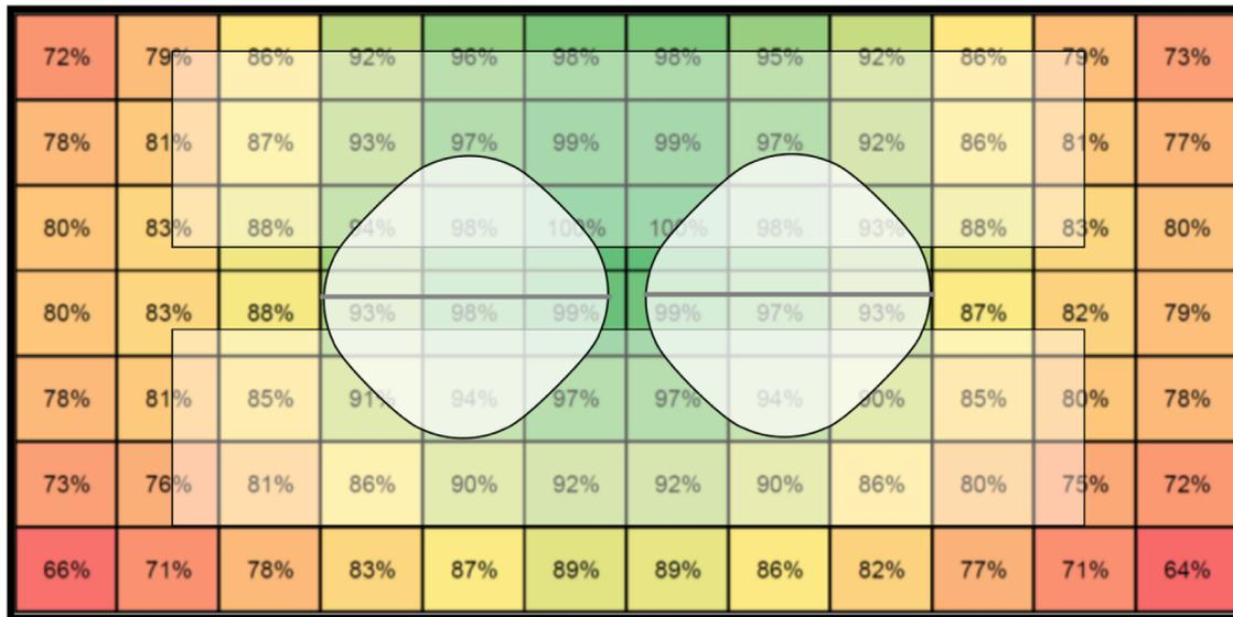
**Figure 1.** Schematic top-down view of the irradiation chamber with decreases of irradiation efficiency in the different areas.<sup>16</sup> The door of the chamber is on the bottom of the figure. The masks are figured in white; the metallic mask holders are figured in transparent white.
