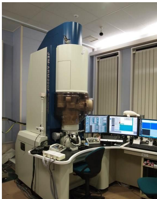
FIG. 1. The appearance of JEM-ARM200F with the cold FEG.
