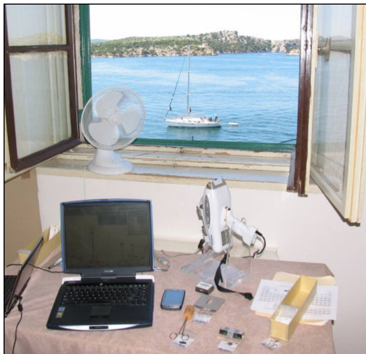
Figure 2. Conducting pXRF analyses of obsidian within a museum in Croatia
