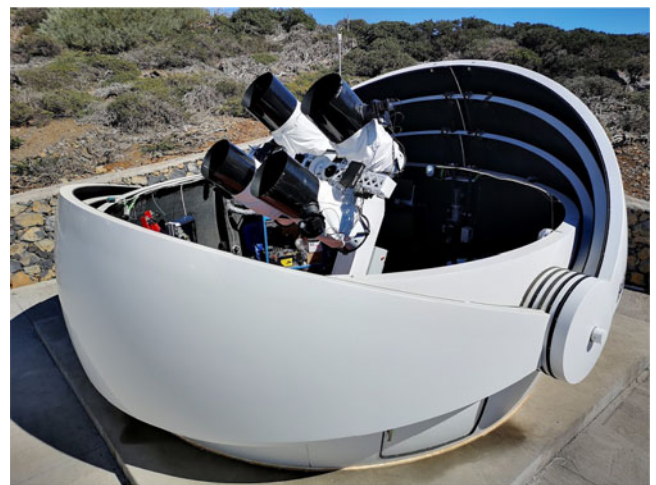
Figure 2. A photograph of the first GOTO mount located on La Palma during its prototype phase when it was equipped with four UTs. Since this photograph was taken, four more UTs have been added to this mount. Image from Dyer (2020).
