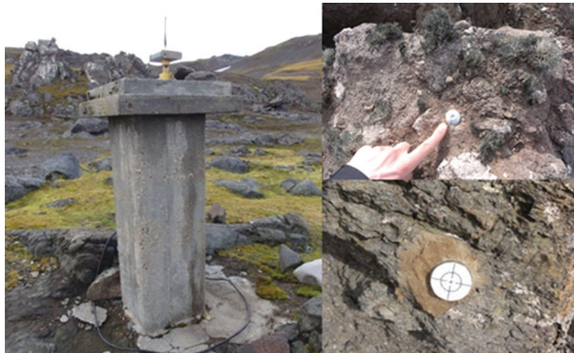
Fig. 1. Methods for control point stabilisation: Jasnorzewski Point on a concrete pillar (left), ground benchmark mounted on the surface of rock outcrops (top right) and benchmarks with a laser-reflecting tape mounted on the sides of rock outcrops (bottom right) (photographs by M.E. Kowalska and M. Rajner).
