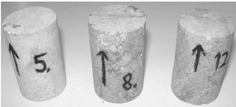
Figure 2.9 Three core plugs with a diameter of 3.81 cm and a height of 5 cm.
