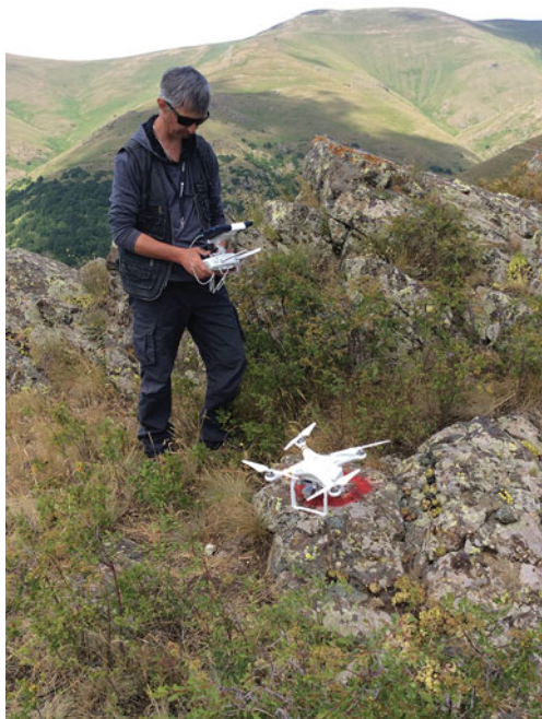
Figure 4. Arshaluys Mkhrtchyan (Project ArAGATS), using Pix4D Collector application on an iPad Mini to program a flight mission for a Phantom 3 Pro drone in order to record a fortress site in the remote hills of the Tsaghkunyats Range, northern Armenia (photograph credit: Ian Lindsay).
