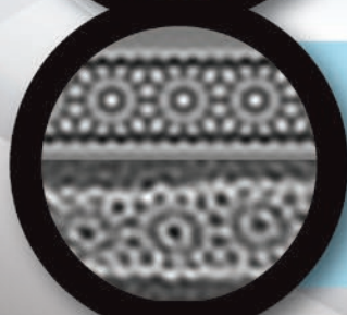
Dr. Miguel Jose Yacaman University of Texas, San Antonio Sample provided by Tour Lab, Rice University Chiral Nanotube with parameters n=10 and m=4 (Simulated and experimental). — 0.5nm
