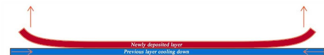
Figure 6. Shrinkage of lower layers and pulling of upper layers up due to cooling.
