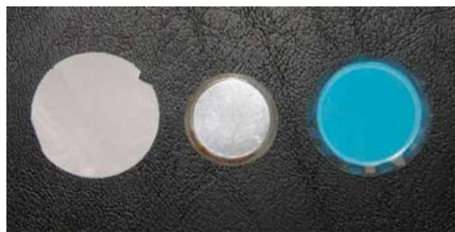
Figure 7. Hydrogen/ \text{CO}_2 separation membranes currently under development: (left) Poly-ionic liquid membrane for \text{CO}_2 removal; (center) multilayered, dense metal hydrogen separation membrane; and (right) copper-based, alumina-supported metal organic framework membrane for \text{CO}_2 separation. (Image courtesy of D. Luebke, B. Howard, and M. Schwartz of the U.S. National Energy Technology Laboratory.)
