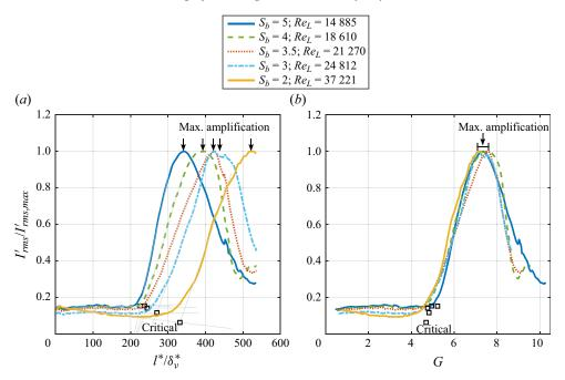
Figure 3. Meridional profiles of r.m.s. of surface temperature fluctuations  $(I'_{rms}/I'_{rms,max})$ , caused by the growth of instability-induced spiral vortices on a rotating cone ( $\psi = 15^{\circ}$ ), represented along (a) scaled meridional length  $l^*/\delta_{\nu}^*$  and (b) Görtler number scale. Squares and downward arrows represent the critical and maximum amplification points, respectively.
