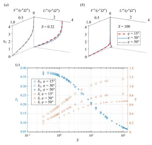
Figure 2. Three-dimensional boundary-layer profiles on rotating cones ( $\psi = 15^\circ$ ,  $30^\circ$  and  $50^\circ$ ) with examples of (a) strong axial inflow S = 0.32 and (b) strong rotation S = 100. (c) Variation of the azimuthal momentum thickness with the local rotational speed ratio S. Here  $\delta_1$  is the momentum thickness in the transformed wall-normal coordinate  $\eta_1$ ;  $\delta$  is the momentum thickness in the scaled wall-normal coordinate  $\eta = z^*/\delta_0^*$ .
