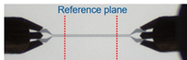
Figure 8. Microscopic image of an on-wafer S-parameter measurement of a CPW transmission line.
