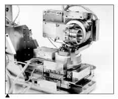
In-Vacuum Submicron Positioning Stage and Controllers: Thermionics Vacuum Products' MicroPositioning Stage and controllers provide vibration-free submicron motion for applications such as SEM, TEM, and PEEM. The piezoelectric in-vacuum motors and encoders are designed for 0.2-µm incremental motion, 0.1-µm resolution, and 250 mm/s velocity. The MicroPositioning Stage is UHV-compatible and can be configured for up to six axes of motion. Contact: sales@thermionics.com; www.thermionics.com.
