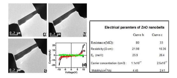
In conclusion, we have shown that the electrical transport properties of the nanobelt could be tuned from the insulating to semiconducting by inducing stress into the nanobelt using an in situ AFM-TEM stage. The semiconducting parameters were retrieved from the experimental I-V curves using the M-S-M model. The structural investigations of the nanobelts show that each nanobelt is single crystalline with hexagonal wurtize structure and grown in the [01\overline{10}] direction.
