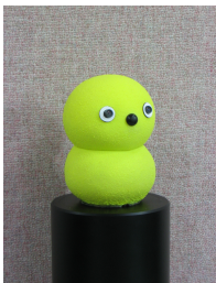
Figure 2.5 Keepon (2003–present), a minimal social robot developed by Hideki Kozima. The robot was later commercialized as an affordable toy. (Source: Hideki Kozima, Tohoku University)
