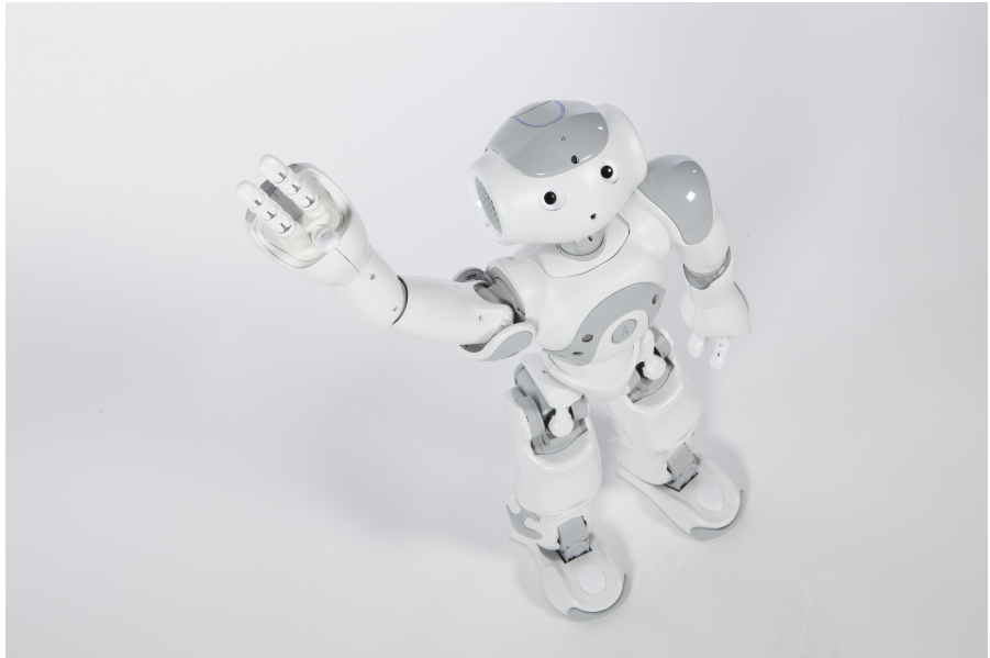
Figure 2.4 Nao (2006–present), a 58-cm-tall humanoid robot, currently the most popular research platform in social robotics.
