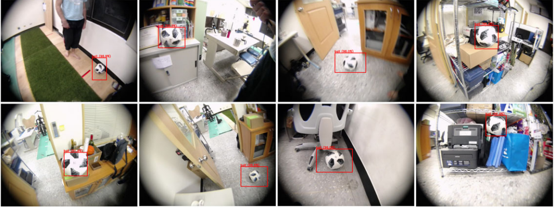
Figure 9. Results of the perception system showcase the robustness in challenging scenarios: around similar colored objects, a cluttered shelf, and blurry images.
