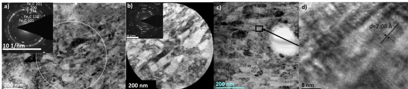
**Figure 1.** TEM images of HPT 316 showing **a)** smaller equiaxed grain regions and **b)** more elongated grain regions with their associated SAED rings. **c)** TEM image of HPT 304 with Cr-rich precipitates and **d)** HRTEM image of the highlighted Cr-rich precipitate in (c).
