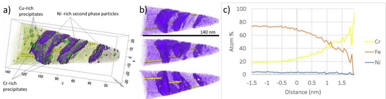
**Figure 2.** **a)** APT data for HPT 304, where Ni-rich precipitates are in blue, Cr-rich precipitates in yellow, and Cu-rich precipitates in green. **b)** View of Cr-rich precipitates from different angles. **c)** Proxigram of the left Cr-rich precipitate seen in **a)** and **b)**.
