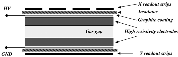
Figure 12.3 Schematics of a resistive plate chamber.
