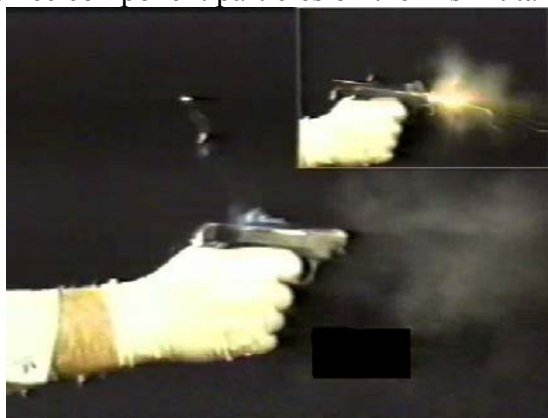
Figure 2. Plume observed around automatic pistol
