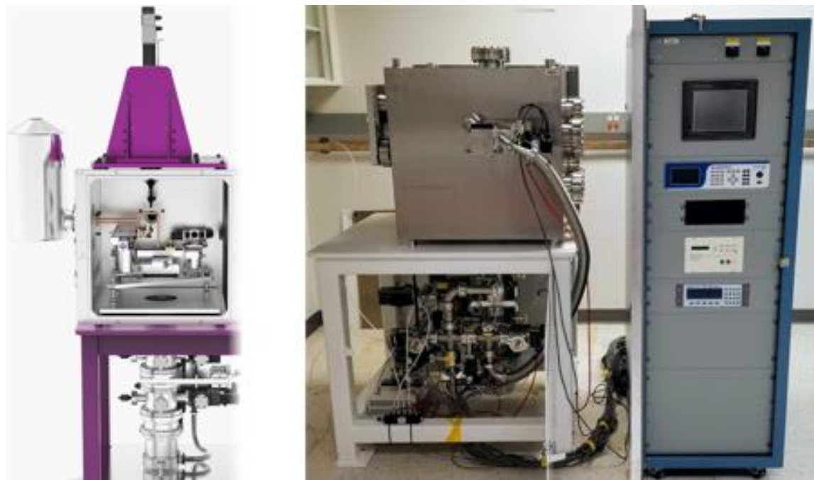
Figure 1. CAD mock-up of the completed C3LM alongside it in its current state of development (including the controllers for the motors, interlocks, and vacuum gauges).
