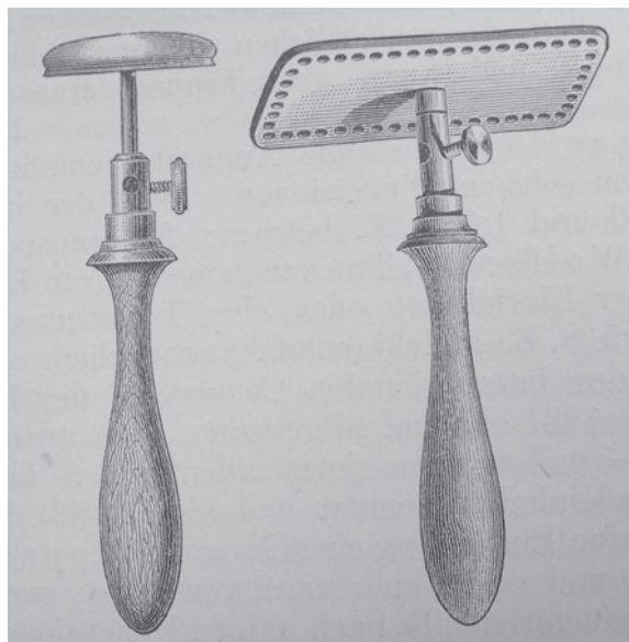
Fig. 2. Plate electrodes with or without hands, the latter used as fixed electrodes (fixed firm to the body), show either round (left) or rectangular (right) application surfaces (source: Lewandowski, 1887, p. 214).
