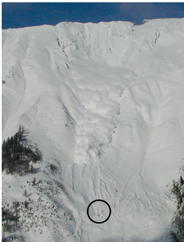
Fig. 1. Avalanche path of the mixed flowing-powder avalanche No. 628 at the Vallée de la Sionne avalanche test site. The 20 m high pylon is marked with a black circle.
