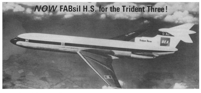
FABsil H.S. the new High Strength Silicone Elastomer has been approved and specified for Cable Identification Markers by Hawker Siddeley Aviation Ltd. and British European Airways Ltd. for use on the Trident Three Jet Airliner. Siegrist's FABsil H.S. Cable markers have Heat Resistance, Elasticity, Tensile Strength, Fire Retardence, and are proof against many fuels, particularly Skydrol 500A. They have many properties not found in any other type of cable marker.
