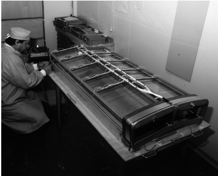
Figure 14.21 Two DELPHI barrel RICH TPC modules. Picture CERN (1986).
