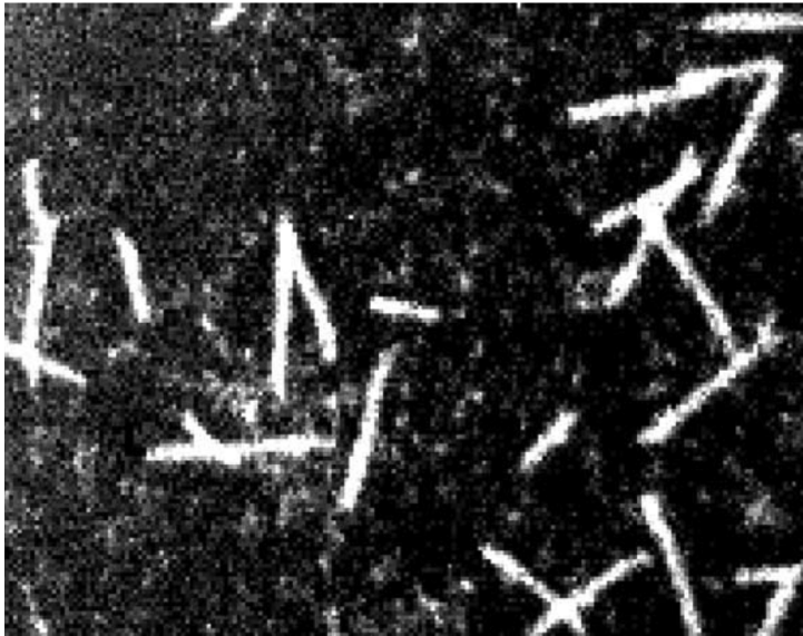
Figure 15.7 Neutron interactions in ^3\text{He} detected with a GEM-based optical imaging chamber (Fraga et al. , 2002). By kind permission of Elsevier.
