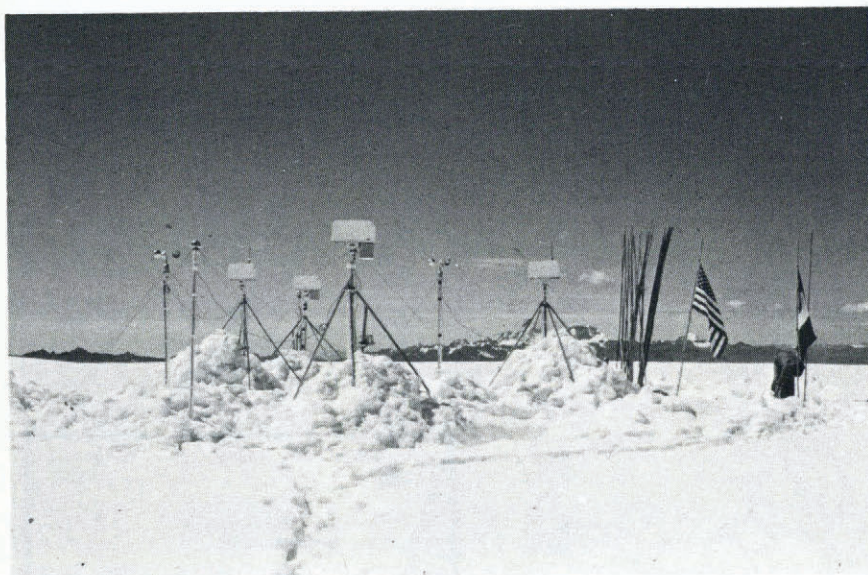
Fig. 4. Automatic meteorological station installation at the summit of the Quelccaya ice cap (5 650 m).
