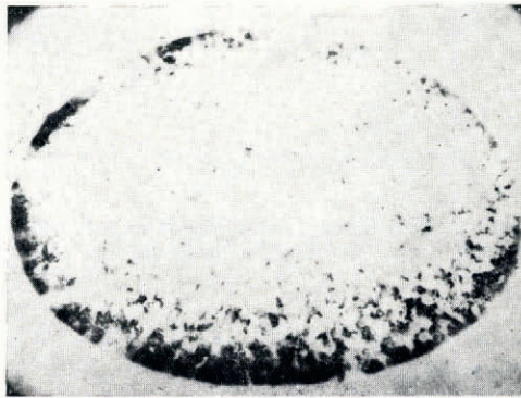
Fig. 6. Photograph of a thin section of a quenched, partially frozen drop with a maximum diameter of c. 0.5 cm; dark areas represent clear ice. (The cut was taken about 0.06 cm from the minor axis.)
