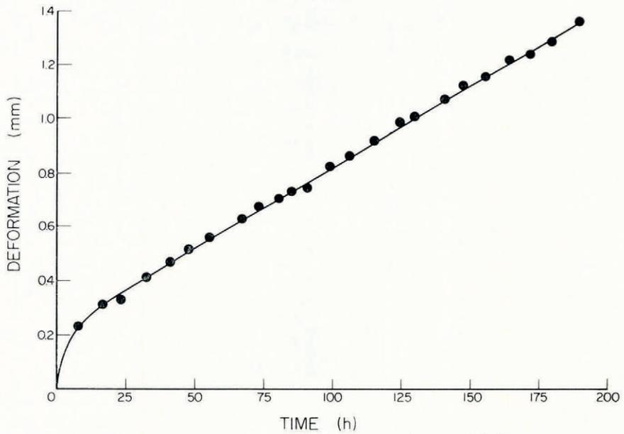
Fig. 4. Typical deformation versus time curve ( $\sigma = 0.58$  bar).
