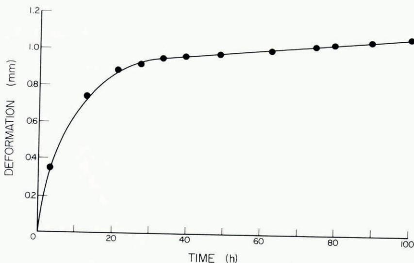
Fig. 3. Typical deformation versus time curve ( $\sigma = 0.1$  bar).
