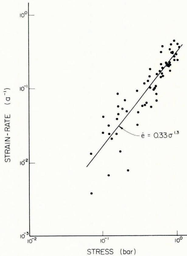
Fig. 5. Stress versus strain-rate.
