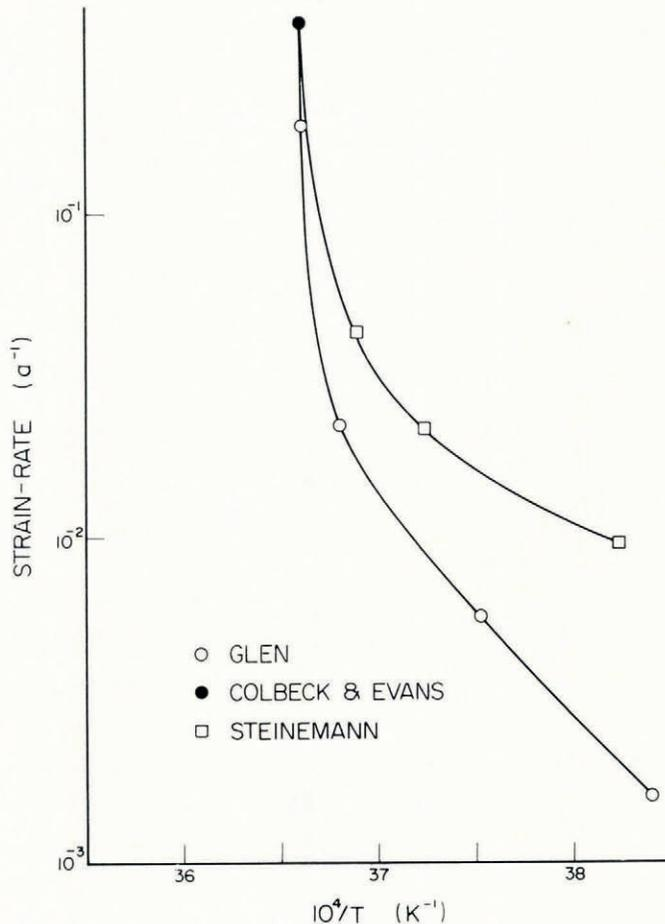
Fig. 8. Strain-rate versus reciprocal of absolute temperature at 1 bar.
