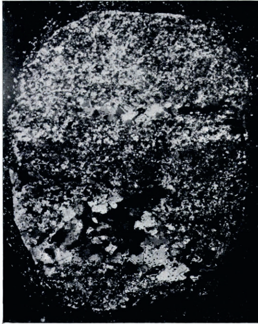
Fig. 4. Thin section of typical amber ice showing coarser-grained clear layers. For scale see Figure 11. (Section A3.2 V2, between crossed polaroids.)
