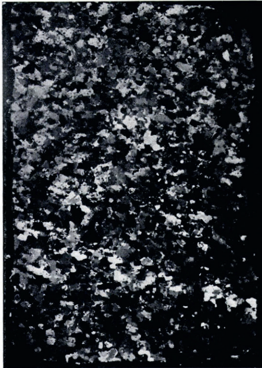
Fig. 2. Thin section of typical white bubbly ice. For scale see Figure 11. (Section B9, between crossed polaroids.)
