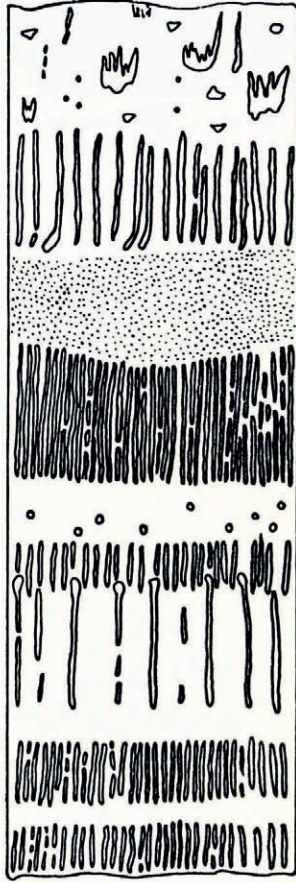
Fig. 20. Sketch of core through a man-made lake. Note migrating bubble clusters and similarities to Figures 18 and 19
