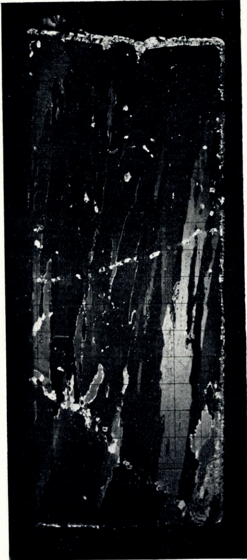
Fig. 10. Vertical thin section of sea ice showing typical sutured crystal boundaries, brine pockets, and also healed fractures indicated by the two light colored diagonal lines of bubble concentrations (ridge core; depth 27.26–27.46 m.; photographed between crossed polaroids, grid lines are 1 cm. apart)
