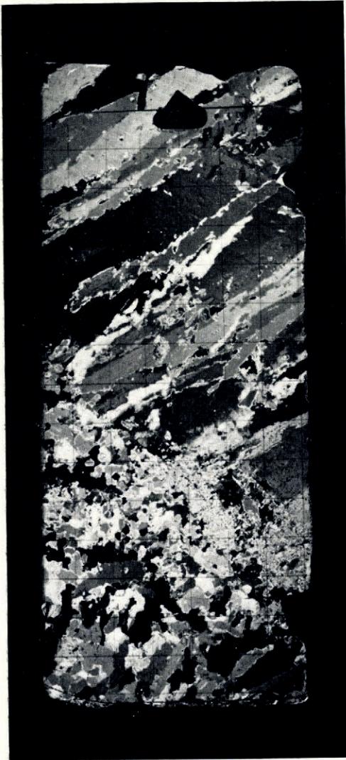
Fig. 13. Horizontal thin section of sea ice in the transition zone with rounded crystal edges (trough core; depth 25.69 m.; photographed between crossed polaroids, grid lines are 1 cm. apart)
