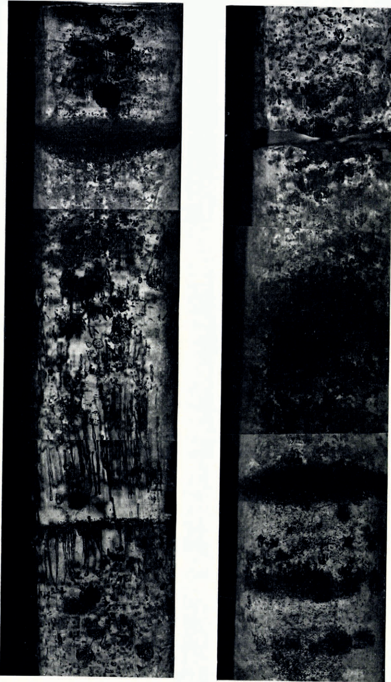
Fig. 13. Section of lake ice showing the typical bubble pattern observed in all lake-ice increments of the core (trough core; depth 5.19-5.98 m.). The top of the core is at the top right; the bottom at the bottom left
