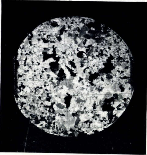
Fig. 8. Horizontal thin section of very fine and fine texture homogeneous sea ice (re-entrant core; depth 9.40 m.; photographed between crossed polaroids, grid lines are 1 cm. apart)
