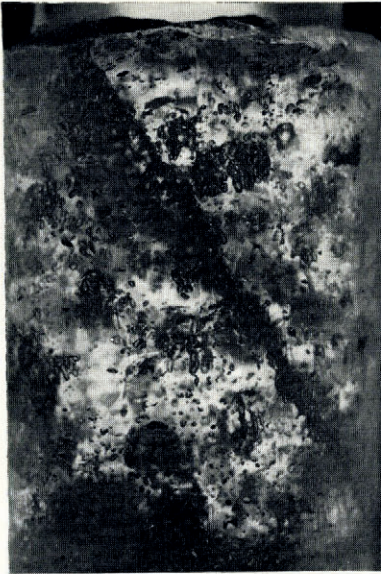
Fig. 16. Bubble plane in lake ice marking a healed fracture (trough core; depth 5.93–6.03 m.)
