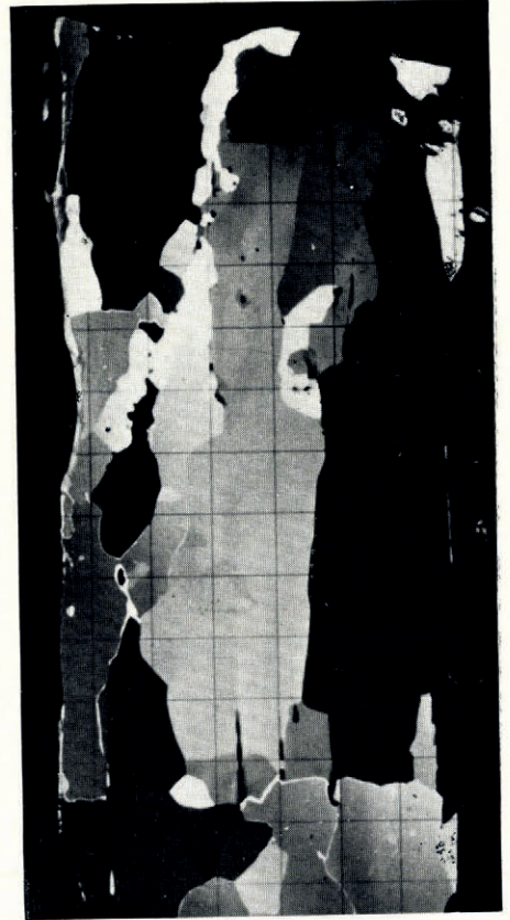
Fig. 7. Vertical thin section of lake ice (trough core; depth 10.25-10.40 m.; photographed between crossed polaroids, grid lines are 1 cm. apart)
