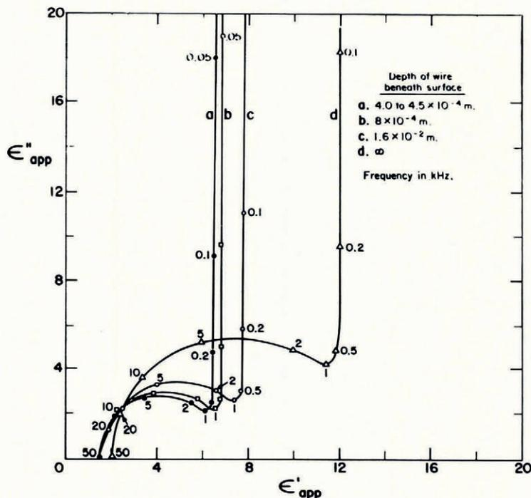
Fig. 3. Cole-Cole plots of the real and imaginary parts of apparent permittivity for wires buried beneath the surface of a cold névé
