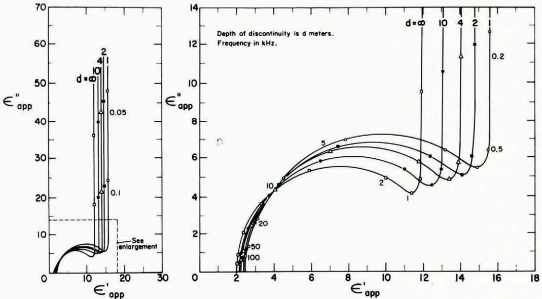
Fig. 5. Cole-Cole plots of the real and imaginary parts of apparent permittivity for cold névé overlying dense warm ice
