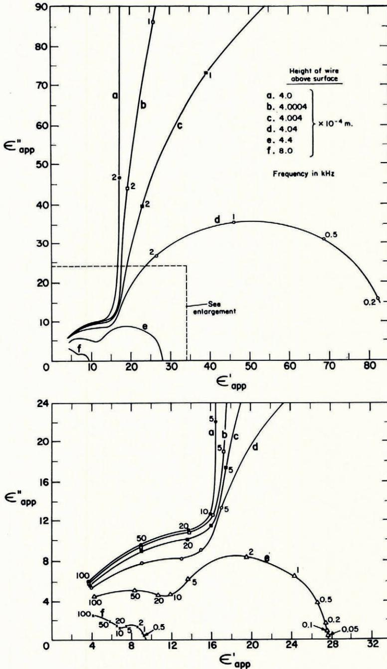
Fig. 2. Cole-Cole plots of the real and imaginary parts of apparent permittivity for wires raised above the surface of a warm wet glacier
