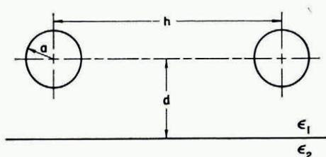
Fig. 1. Geometry of the electrodes
