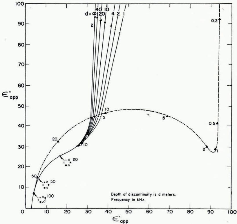
Fig. 4. Cole-Cole plots of the real and imaginary parts of apparent permittivity for warm wet ice overlying deep pure dense ice. Superimposed is a plot for deep ice alone
