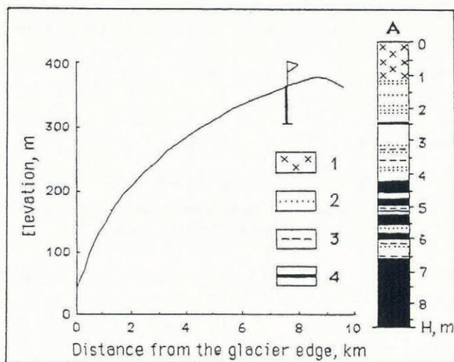
Fig. 1. Surface-elevation profile of the northern slope of the Looney ice cap and stratigraphy of firn layers from a core near the deep-hole site (A): 1; snow 2–4, ice layers with a thicknesses less than 1 cm, 1 cm and more than 1 cm, respectively.
