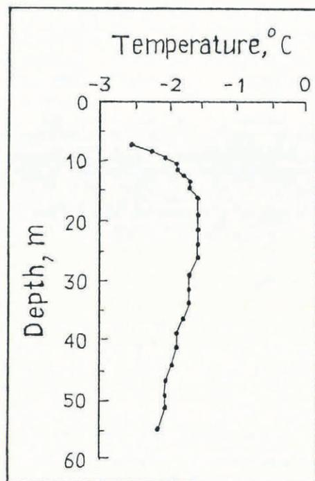
Fig. 2. Temperature distribution in the Looney ice cap.
