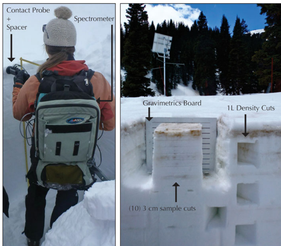
Fig. 3. (Left) Picture demonstrating contact spectroscopy; typically the snow pit would be covered by a tarp to reduce outside illumination. (Right) Picture of snow pit showing density cuts and gravimetric sampling, the 3 cm cuts are made using a white powder coated saw (not pictured).
